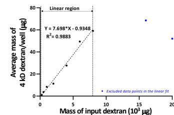
Dextran delivery to individual wells can be modulated by varying the exposure duration while maintaining a constant dextran input concentration of 8 mg/mL.
